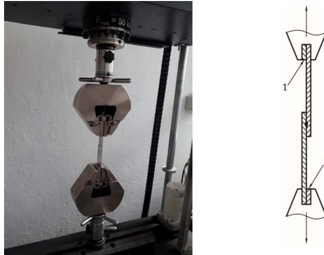
Figure 4. Specimen prepared for testing.
