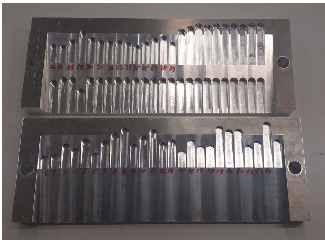
Figure 7. Workpiece after experimentally defined stability lobe diagram
