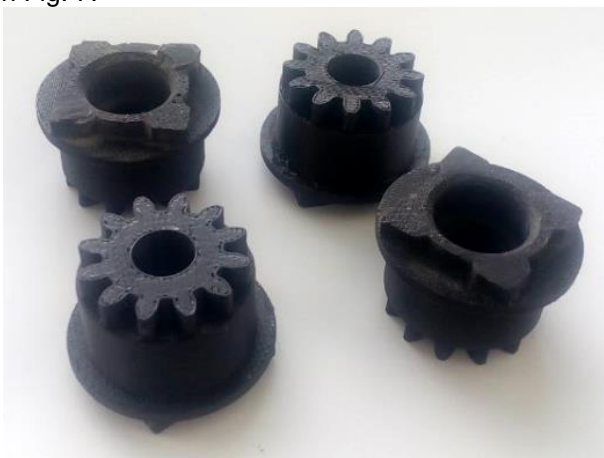
Fig.7 Small batches of gears made in the integrated process of additive manufacturing technology and vacuum casting
