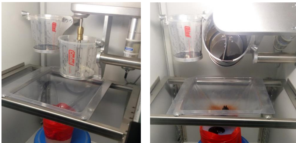
Fig. 6 The casting process in a vacuum chamber MK-mini
