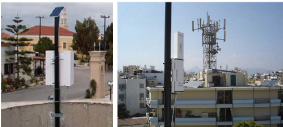
Figure 3. Examples of monitoring stations: EE4070-WB RMS station at Koskinou, Rhodes (left) and MCE-410 RMS station at Heraklion, Crete (right)
