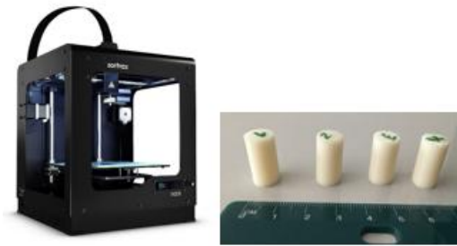
Figure 3. (a) 3D printer Zortrax M200; (b) Specimens
