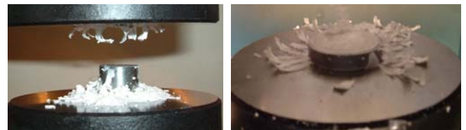
Figure 9 – (a) Picture of specimen before upsetting process, (b) Picture of specimen after upsetting process [3]
