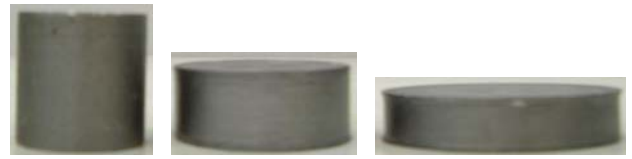
Figure 8 – Pictures of specimen in typical phases during cylinder upsetting using method Rastegajev
